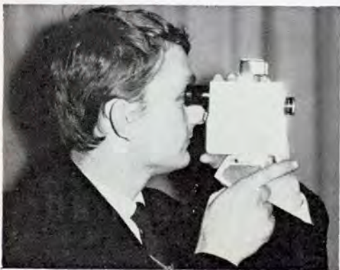
Mr Belcher using his Prince camera fitted with pistol grip and trigger release. The eye-piece was made from an eye-bath and a miniature exposure meter is fitted on top.
