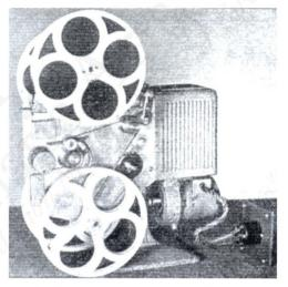
Baird Cine-Soundmaster 1st version bolted to a Kodascope 8mm 8–46 projector
