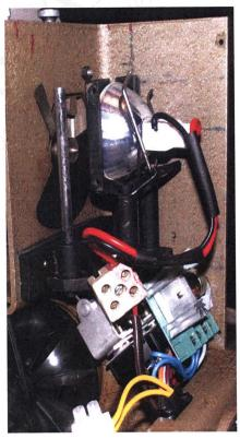
bulb. It slides up and down by means of a hollow tube affixed to the dowser. A handle is fitted to the top of the dowser and protrudes from the top of the lamp house
