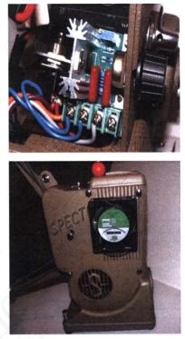
In order to keep the lamp cool without the motor running I decided to add an auxiliary fan The one that I used came from eBay - 80x80x25mm with plastic blades metal frame and Axial cooling fan AC 220/240volt 0 07amp 13watt The cost was about £14 The only drawback was that I had to drill a hole in the Specto but I do have another one if ever I should have to remake the projector
