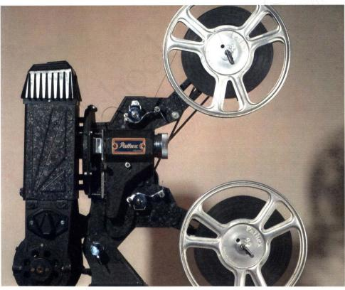
Here we have the well known 200B nine five silent projector suitably laced and showing the feed and take up spools to good effect with film. Note the nameplate that states it as being Pathex. The reason for this is fully explained in the excellent article by Bryan Pearce in this issue appearing from page 22 with appropriate pictures to accompany the text. All were taken by Bryan along with this cover picture.
