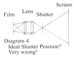
film The two point sources shown in Diag 4 would of course focus as two separate images on the shutter Similarly rays from a fully illuminated film frame would all focus to yield its complete image on the shutter - or better still on a screen if placed at the same location!
