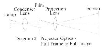
fact diagrams showing the action of a camera lens usually resort to this simple artifice to show why it delivers an inverted image to the film. It also helps to explain why a simple pinhole can also act as a lens albeit of very small aperture!
