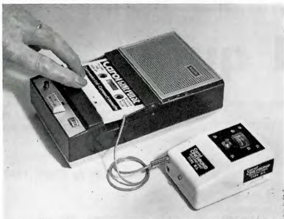
The Cinepulse Cassette with the Carol R1 tone generator unit and a standard Philips cassette recorder.
