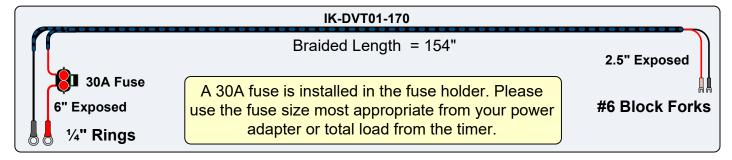
The IK-DVT01-170 Wire Kit provides a 10 gauge power feed harness from the battery to the DVT01-C Timer and to a laptop power adapter. An installation kit with a spare fuse, pre-terminated wires, and spare terminals is also provided.
