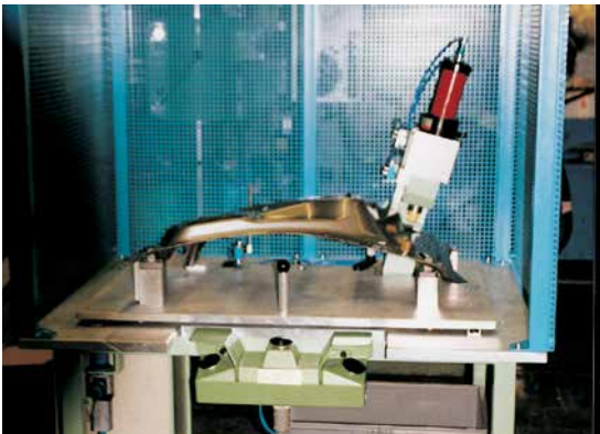
Device for holes Ø 8 in sheet metal
